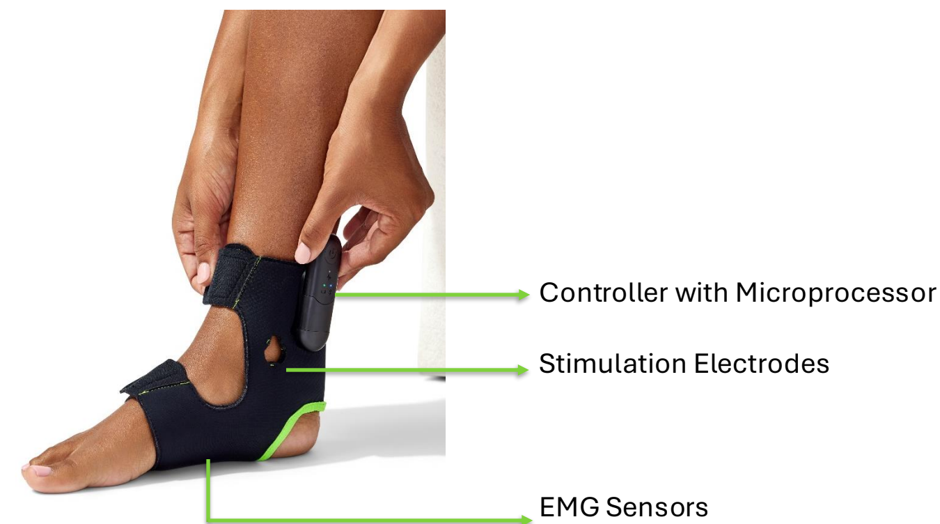
Figure 2: The wTNM system with PCL stimulation and integrated garment with built-in electrodes shown on a patient's foot.
